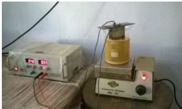
Fig. 2. Experimental Set up of Electro Fenton process
